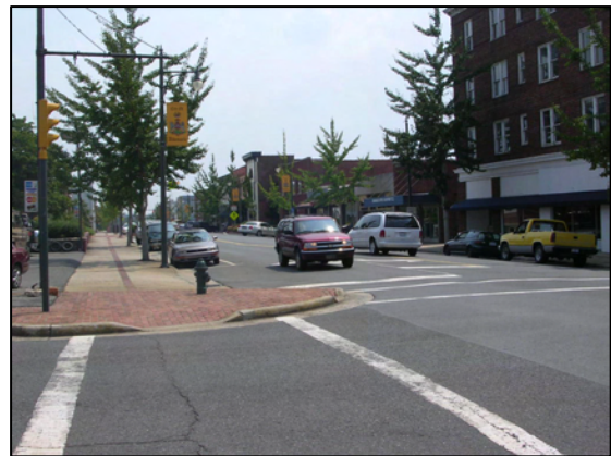
Pedestrians have less road width to cross when there is a curb extension and cars are forced to slow down to make right turns.
